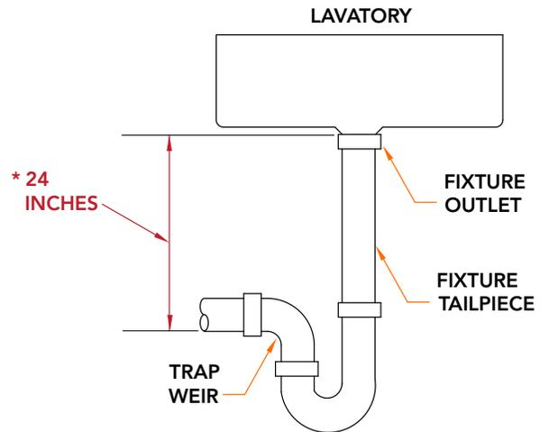
\*MAXIMUM DISTANCE FROM FIXTURE OUTLET TO TRAP WEIR
