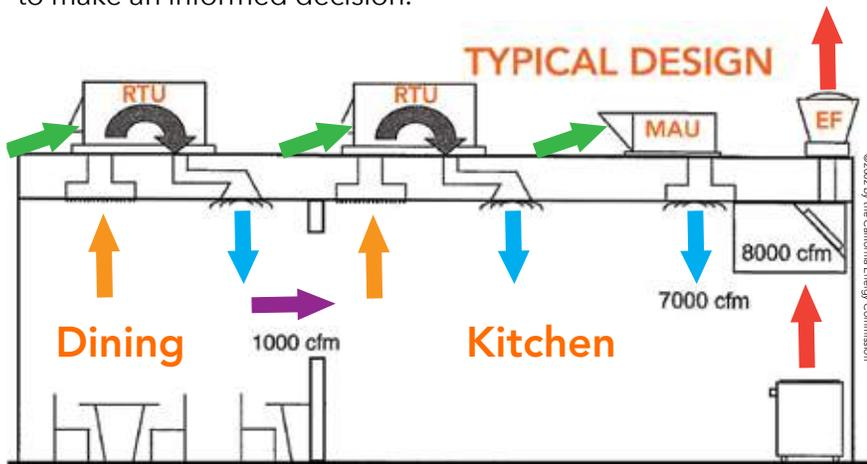
Figure 7. Typical HVAC equipment arrangement for a restaurant.
