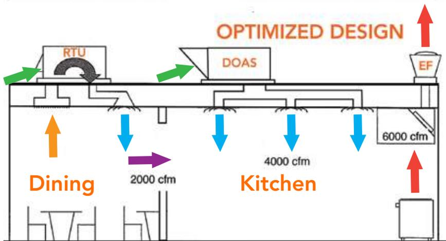
Figure 8. Optimized HVAC equipment arrangement for a restaurant.
