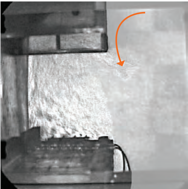
Figure 5. Schlieren image shows the thermal plume being pulled outside the hood by the air discharged from a 4-way diffuser.
